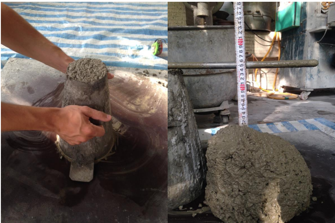
Fig. 5 Slump test of fresh concrete
