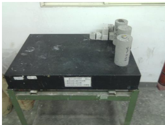
Fig. 3-21 Horizontal table for the smoothness verification of sample ends
