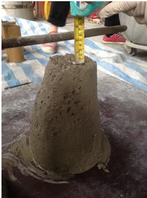
Fig. 3-1 Slump test of fresh concrete
