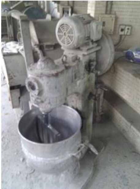
Fig. 3-18 Big concrete mixer
