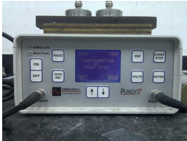
Fig. 3-24 Ultrasonic Pulse Velocity Meter “Pundit 7”
