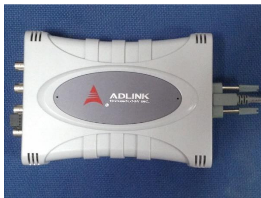
Fig. 3-28 Data acquisition system AD-Link
