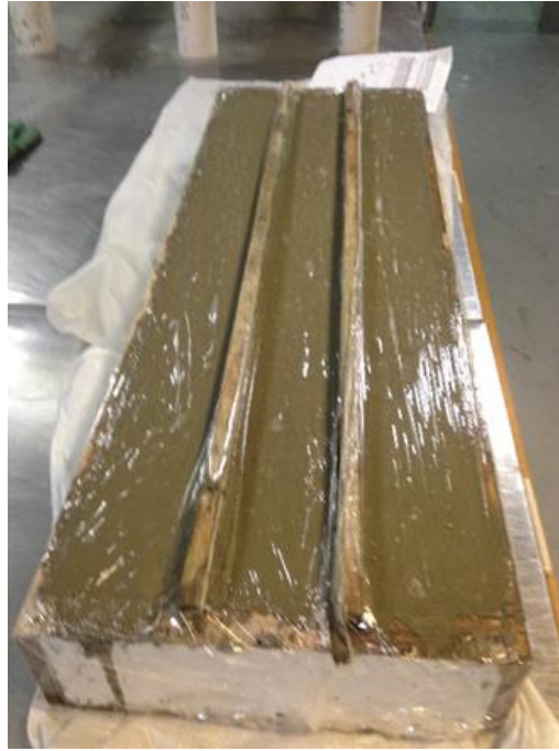
Fig. 3-2 Concrete beam specimens
