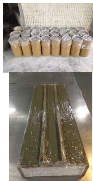
FIGURE I. CASTING OF CONCRETE SAMPLES
