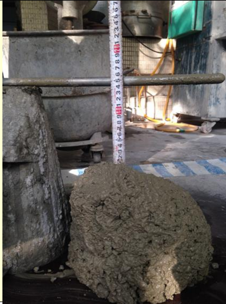
Fig. 5 Fresh concrete slump test: 140 mm
