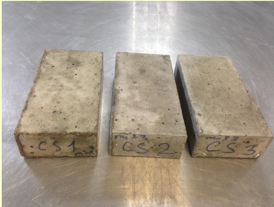
Fig. 4 Concrete blocks 120x80x40 mm for internal friction test
